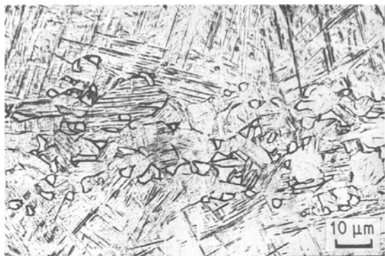
Figure 2 Microstructure at 1050° C for 1 h, water-quenched.
